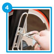
Using the multi tool attach the bottle holder to the frame
